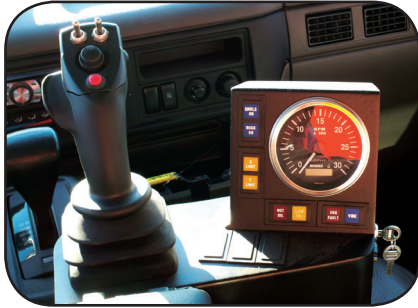
In-cab patching controls.
