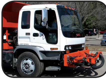
Boom folds flush with front bumper.
