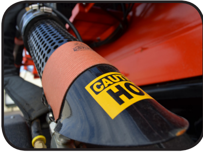
Vent-Flo Nozzle with optional Heater.
